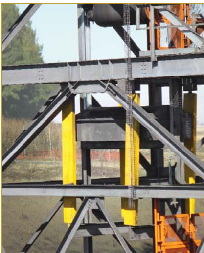
Closer view of the yellow Technogrids® with the counter weight hanging in between them.
